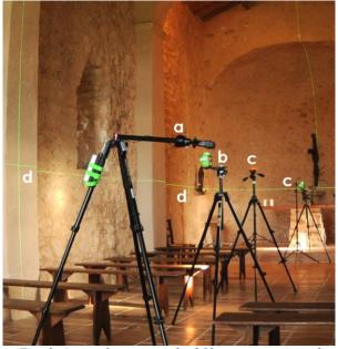
Fig. 3. A sample setup: **a** the 360 camera; oriented horizontally, **b** a laser level, **c** tripods on which acoustic devices wuill bemounted, **d** intersection of laser beams on the enveloppe.
