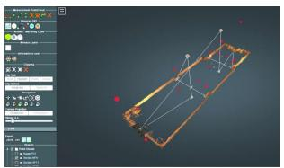
Fig. 5. The polyline that corresponds to the scaling protocol (DXF outputted by the Leica Disto), represented inside the Potree point cloud renderer.
