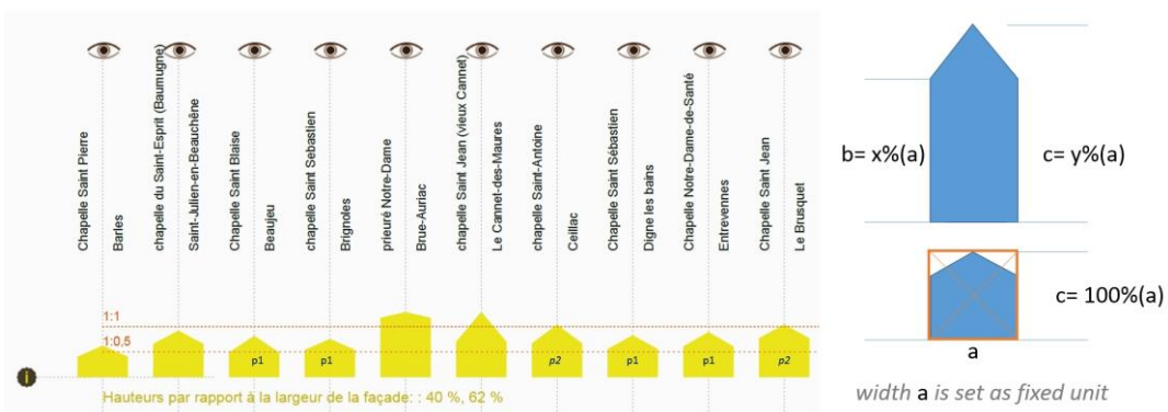
Fig 6 Left, the visual formalism dedicated to the comparative analysis of proportions of facades (partial view). Note for instance patterns p1 and p2, and in contrast the four remaining edifices. Right, the making of the figure: a is a fixed unit, b corresponds to dimension H1 and c to dimension H2 as defined in Fig5, expressed in proportion to W1. An edifice with a width and
