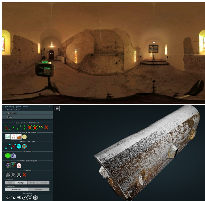
Figure 11. A case found to be critical for IBM (Saint-Roch chapel, Les Méés). Top, a stitch showing the predominance of white surface in the edifice. Bottom, the reconstruction, combining the photogrammetric model (brown points) and the laser scanner's output (white points).
