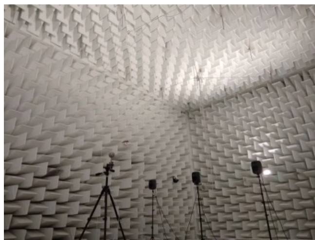
Figure 9. The Eigenmike 32 and speakers positioned for reference measurement in an anechoic room.
