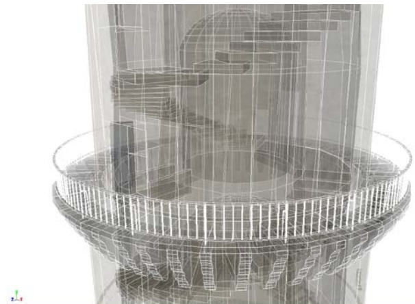
Figure 5: A partial view of a 3D model of the signal light tower, showing the balcony on level 3 and the spiral staircase. Full credits will be given to authors of these graphics in a non-blinded version of this paper
